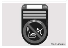
If the front-passenger seat of your vehicle is not equipped with the automatic front-passenger front airbag deactivation system, this is indicated by a special sticker. The sticker is affixed to the side of the dashboard on the front-passenger side. The sticker is visible when you open the front-passenger door.
