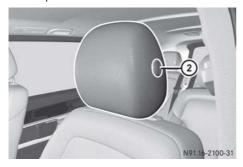
➤ To adjust the height: turn the key in the ignition lock to position 2.
