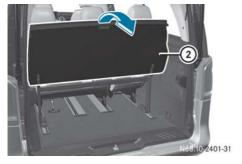
Make sure that the luggage compartment partition is always folded down when the vehicle is moving.
