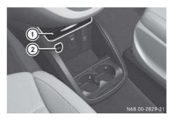
Socket on the centre console (example: centre console with cover)
