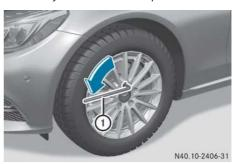
▶ Loosen the wheel bolts on the wheel to be changed in an anti-clockwise direction by about one turn using wheel wrench ①. Do not remove the wheel bolts.
