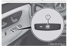
► To activate/deactivate: press button (1). If the indicator lamp on the button is lit, operation of the rear-compartment electrical hinged windows is disabled. Operation is then only possible using the buttons in the driver's door.
