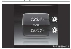
► Press and hold the <u></u> steering wheel button until the Trip menu with trip meter (1) and total distance (2) appears.
