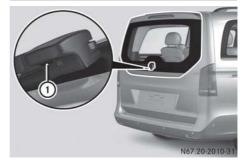
If your vehicle is equipped with the EASY-PACK tailgate, the [31] button of the key must be programmed to open the rear window (⊳ page 84).
