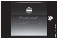
If a no entry sign or roundabout sign is passed, warning message ① is shown in the display if Traffic Sign Assist detects that the vehicle is travelling in the wrong direction. An additional warning tone sounds. Immediately check the direction in which you are driving. Only by doing so are you able to avoid any potential risk to yourself and other road users.
