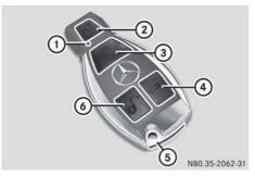
Key (example: vehicle with EASY-PACK tailgate and/or rear window which can be opened separately)
