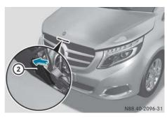
▶ Reach into the gap, push lever ② of bonnet catch to the left and lift the bonnet. If you open the bonnet approximately 40 cm, the bonnet is opened and held open automatically by the gas-filled strut.
