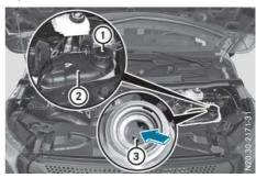
Example: cap and coolant expansion tank
