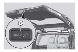
▶ To close: press the ② closing button in the tailgate and step out of the swinging range of the tailgate.
