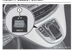
Push AGILITY SELECT switch ① up or down until the desired transmission program is selected.
