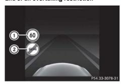
A maximum permitted speed of 60 km/h ① applies. The overtaking restriction no longer applies ②. The crossed-out no overtaking traffic sign is displayed for five seconds.
