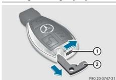
▶ Slide release catch (1) in the direction of the arrow and, at the same time, remove emergency key element (2) from the key completely.
