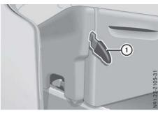
(1) Release handle for seat fore-and-aft adjustment
