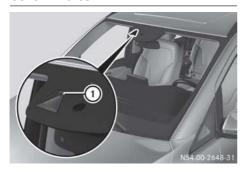
Traffic Sign Assist shows speed limits and overtaking restrictions in the display. If you drive into a section of road in the wrong direction, it will warn you visually and acoustically. Traffic Sign Assist detects traffic signs with camera system ① attached behind the top of the wind-screen. The data and general traffic regulations
