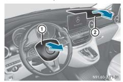
Driver's airbag (1) deploys in front of the steering wheel. Front-passenger front airbag (2) deploys in front of and above the glove compartment and centre console.
