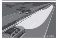
**Active:** if you are driving at speeds above 110 km/h and do not make any large steering movements for at least 1000 m or if you are driving at speeds above 130 km/h.
