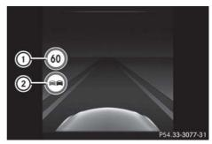
A maximum permitted speed of 60 km/h (1) and an overtaking restriction (2) apply.
