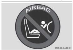
If it is absolutely necessary to fit a rearward-facing child restraint system to the front-passenger seat, always make sure that the front-passenger front airbag is disabled. Only if the PASSENGER AIR BAG OFF indicator lamp is lit continuously (>> page 41) is the front-passenger front airbag disabled.
