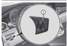
The headlamp range control allows you to adjust the cone of light from the headlamps to suit the vehicle load. The cone of light changes if the seats are occupied or if the load compartment is loaded or unloaded. This can impair visibility and dazzle oncoming traffic.
