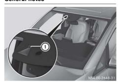
Lane Keeping Assist monitors the area in front of your vehicle by means of camera ① at the top of the windscreen. Lane Keeping Assist detects lane markings on the road and can warn you before you leave your lane unintentionally.
