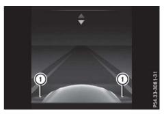
When Blind Spot Assist is activated, the display in the assistance graphic shows grey radar waves propagating backwards next to the vehicle. Above a speed of 30 km/h, the colour of the radar waves in the assistance graphic changes to green ②. Blind Spot Assist is then ready for use.
