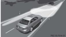
You can use this function to set the headlamps to change between dipped beam and main beam automatically. The system recognises vehicles with their lights on, either approaching from the opposite direction or travelling in front of your vehicle, and consequently switches the headlamps from main beam to dipped beam.
