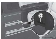
▶ Pull lever ⑤ on the front or rear side of the folding table upwards and push the folding table backwards.
