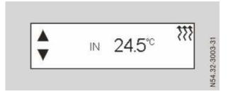
► Use the or button to set the desired temperature between 10 °C and 40 °C.
