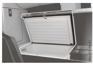
The coolbox is located next to the gas cooker is in the kitchen cupboard. The lid of the coolbox is held in the open position.
