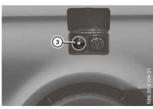
The filler neck for fresh water tank (3) is located behind the service flap in the rear area of the vehicle on the driver's side.
