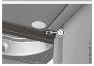
The interior lamps are fitted on both sides beside the roof stowage box and are switched on/off individually. The interior lamps are powered by the additional battery.
