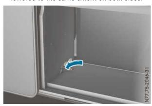
If the electrics of the electric pop-up roof malfunction you can no longer close the pop-up roof normally. However, the pop-up roof can still be closed by emergency operation. The button for activating the emergency operation is in the cupboard under the gas cooker behind the sidewall on the left-hand side.
