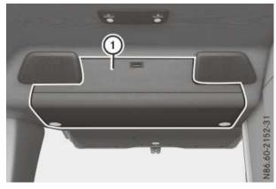
Folding roof stowage box ① is located in the rear area. The flap is secured with a furniture fastener.
