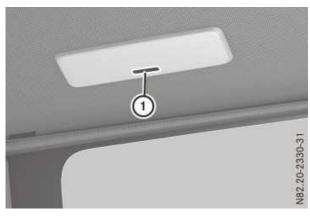
The LED lamps are located on both sides of the vehicle between the B and C-pillars in the roof frame. Both LED lamps can be switched automatically or manually. You can also dim the LED lamps in three levels.
