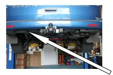
On the chassis behind the bumper you will find an M8 bolt going through two chassis members, remove this bolt. You will need to put a small slot approx 75mm x 20mm in the plastics and feed the mounting bracket through, line up and use the bolt to secure the fill point in place.
