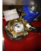
Secure the junction box provided internally in the vehicle and run the two cables from the tank to the junction box. Make the connections as indicated on the board. Bring your 12v DC feed from your leisure system into the centre block.
