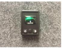
The GASTORE control is microprocessor controlled, on first switching the unit on using the left button you should see the GREEN led's illuminate in a sequence whilst it carries out a self test. This should then leave a single RED led illuminated assuming the tank is empty. During this first 2 seconds the controller is supplying 12v@1A to the solenoid to open it, after this 2 seconds, and now
