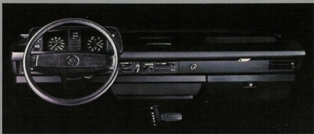
Fully padded instrument panel is ergonomically designed to place all controls within easy reach of the driver.
