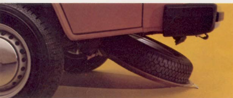
Up-front, under-floor spare tire storage—more room inside.
