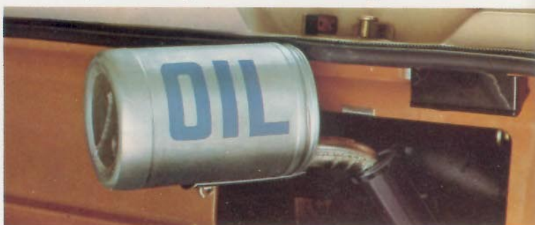
Oil filler neck slides up for easy access.
