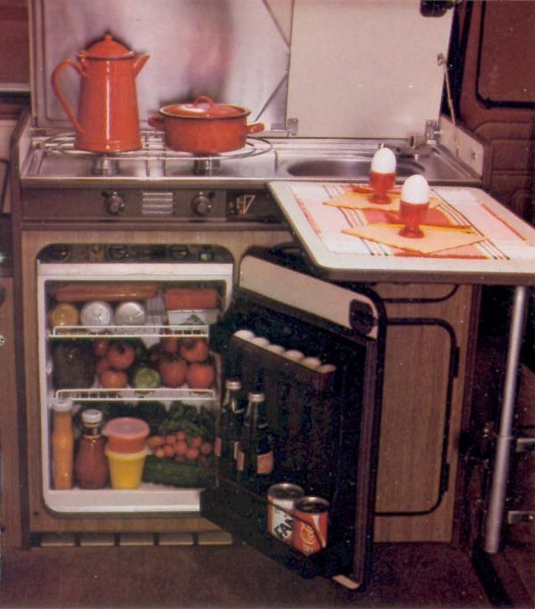
Model P27 has a 3-way refrigerator and a 2-burner cookstove.
