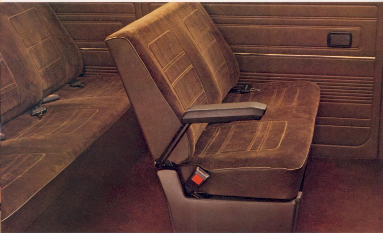
Center seat in Van Dyck cloth. Seat is easily removed when you need extra cargo room, and re-installed in minutes.
