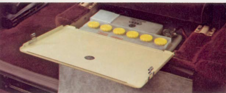
Easy battery access under passenger seat.
